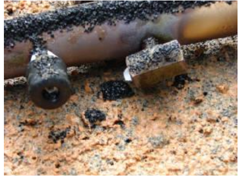
Nozzles and Sweep Parts Which Were Found Needing Maintenance During an Assessment
