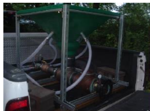
Eductor Ready to be Unloaded to Begin Adding Media to Filter
